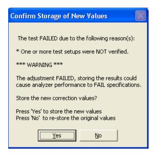
This error message occurs because the 3 GHz RF Assembly Adjustment portion of the LO Amplitude Adjustment test was not performed. Click "Yes" to store the new values. After you click yes, the following message appears on the PC screen:
