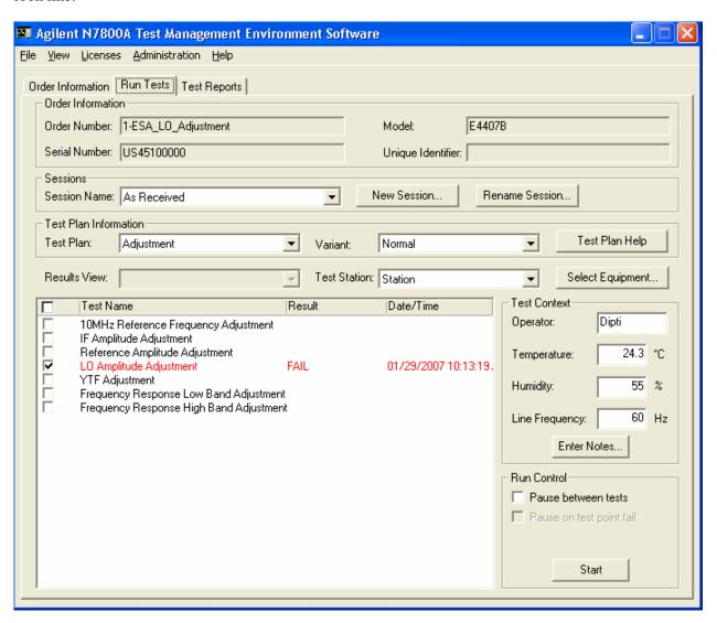
The LO Amplitude adjustment test result appears as Fail because the 3 GHz RF Assembly Adjustment portion of the LO Amplitude Adjustment test was not performed. Ignore the fail message and continue with your tests.
